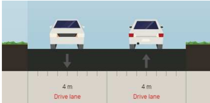
Figure 4-2. Braeside Avenue - Existing Cross-Section
