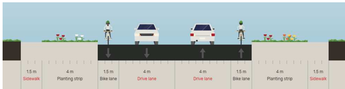
Figure 4-1. Alta Vista Drive - Existing Cross-Section
