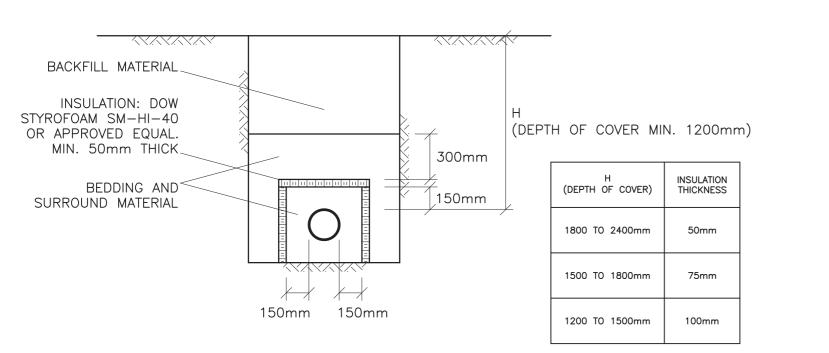
INSULATE WATERMAIN AS INDICATED AND WHERE DEPTH OF COVER IS LESS THAN 2400mm. PROVIDE A MINIMUM 1200mm COVER CENTER INSULATION OVER PIPE. JOINTS BETWEEN SHEETS OF INSULATION SHALL BE STAGGERED.
