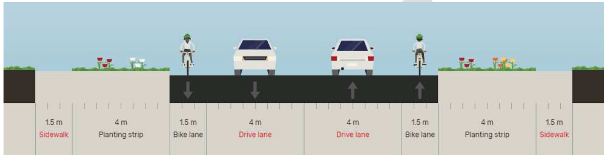
Figure 4-1. Alta Vista Drive - Existing Cross-Section
