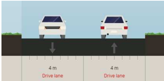
Figure 4-2. Braeside Avenue - Existing Cross-Section
