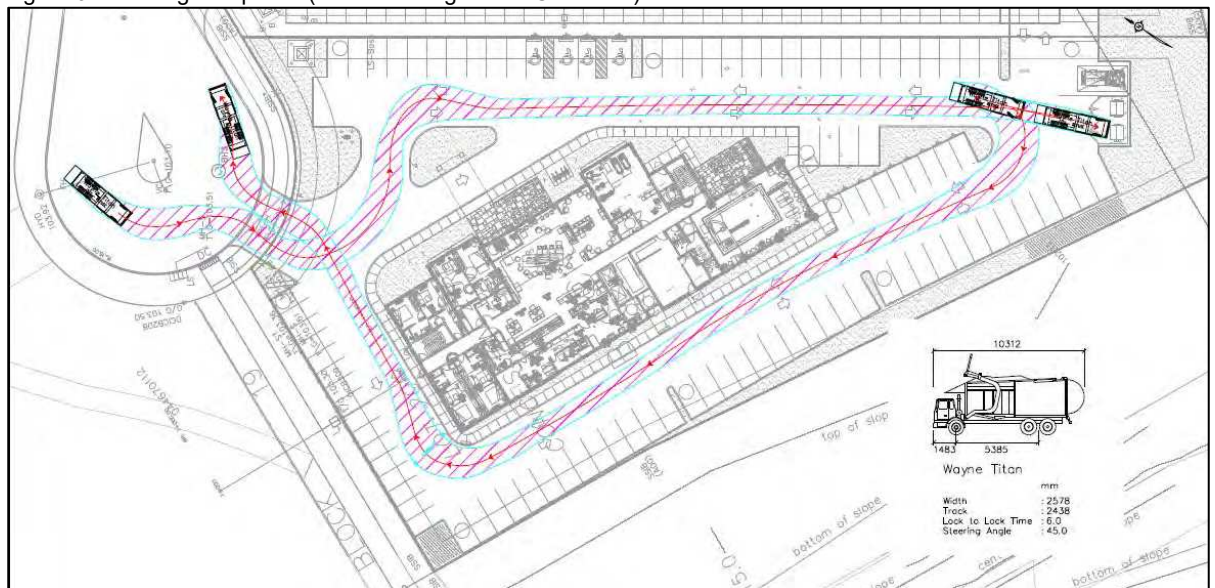
Figure 6 – Turning Templates (Front-Loading Waste Collection)
