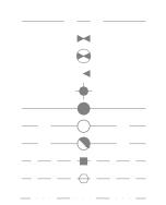
EXISTING WATERMAIN EXISTING VALVE AND VALVE BOX EXISTING VALVE CHAMBER EXISTING REDUCER EXISTING FIRE HYDRANT EXISTING SANITARY SEWER EXISTING STORM SEWER EXISTING CATCHBASIN MANHOLE EXISTING CATCHBASIN EXISTING SUBDRAIN CATCHBASIN
