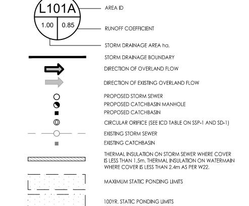
CIRCULAR ORIFICE (SEE ICD TABLE ON SSP-1 AND SD-1)
