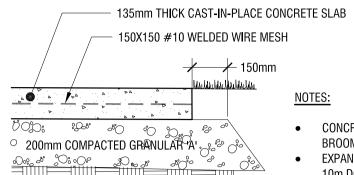
• CONCRETE TO BE 30MPa (4000 PSI) WITH 5-7% AIR ENTRAINMENT AND LIGHT
