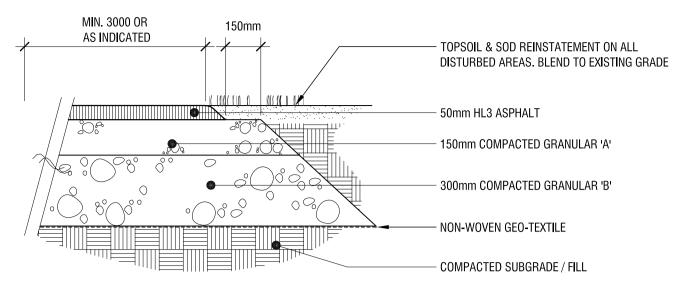
CROSS SLOPE PATHWAYS IN DIRECTION OF NATURAL DRAINAGE AND CROWN / CROSS SLOPE OTHER PAVED SURFACES TO PROVIDE POSITIVE DRAINAGE
