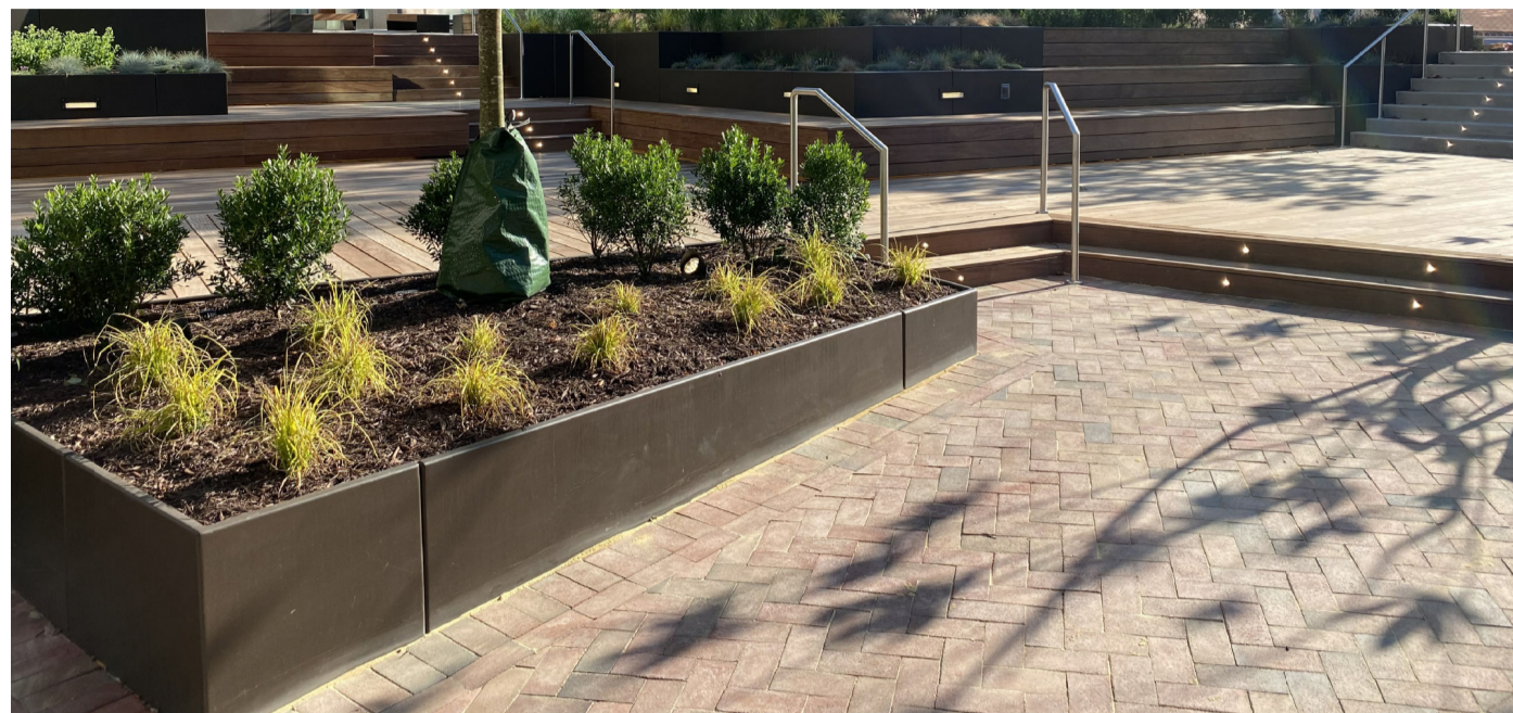
1 BOTTOMLESS RAISED PLANTER IN CORTEN FINISH L4 n.t.s.
