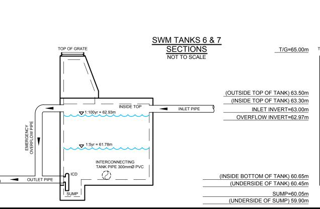
c/w ALUMINIUM LADDEF TOP OF GRATE (OUTSIDE TOP OF TANK) 63.50m (INSIDE TOP OF TANK) 63.30m INLET INVERT=63.00m OVERFLOW INVERT=62.97m RUNGS ON WEST WAL (INSIDE BOTTOM OF TANK) 60.65m (UNDERSIDE OF TANK) 60.45m SUMP=60.05m
