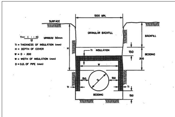
NOTES: -FOR STORM INSULATION USE AN X VALUE OF 2000 IN THE ABOVE "TI" EQUATION. -FOR SANITARY INSULATION USE AN X VALUE OF 2500 IN THE ABOVE "TI" EQUATION. -FOR WATERMAIN INSULATION USE AN X VALUE OF 2400 IN THE ABOVE "TI" EQUATION. -INCREMENTS OF INSULATION THICKNESS SHALL BE ADJUSTABLE TO 25mm. -STAGGER JOINTS OF MULTIPLE SHEETS. -ALL DIMENSIONS ARE IN MILLIMETERS UNLESS SHOWN OTHERWISE.
