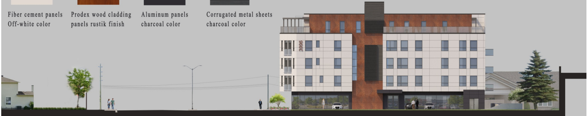
SOUTH WEST ELEVATION
