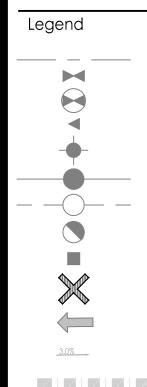
EXISTING WATERMAIN EXISTING VALVE AND VALVE BOX EXISTING VALVE CHAMBER EXISTING REDUCER EXISTING FIRE HYDRANT EXISTING SANITARY MH AND SEWER EXISTING STORM MH AND SEWER EXISTING CATCHBASIN MANHOLE EXISTING CATCHBASIN REMOVAL ITEMS DIRECTION OF EXISTING OVERLAND FLOW FLOW DIRECTION AND GRADE OF EXISTING GROUND
