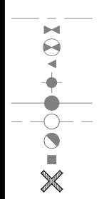
EXISTING WATERMAIN EXISTING VALVE AND VALVE BOX EXISTING VALVE CHAMBER EXISTING REDUCER EXISTING FIRE HYDRANT EXISTING SANITARY MH AND SEWER EXISTING STORM MH AND SEWER EXISTING CATCHBASIN MANHOLE EXISTING CATCHBASIN
