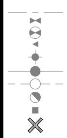
EXISTING WATERMAIN EXISTING VALVE AND VALVE BOX EXISTING VALVE CHAMBER EXISTING REDUCER EXISTING FIRE HYDRANT EXISTING SANITARY MH AND SEWER EXISTING STORM MH AND SEWER EXISTING CATCHBASIN MANHOLE EXISTING CATCHBASIN **REMOVAL ITEMS**
