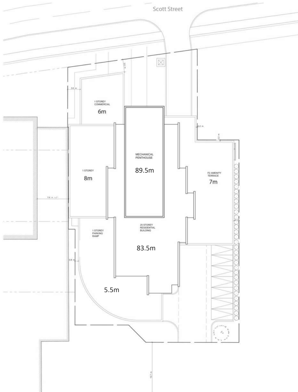
Figure 5.1: Roof Heights of Proposed Building
