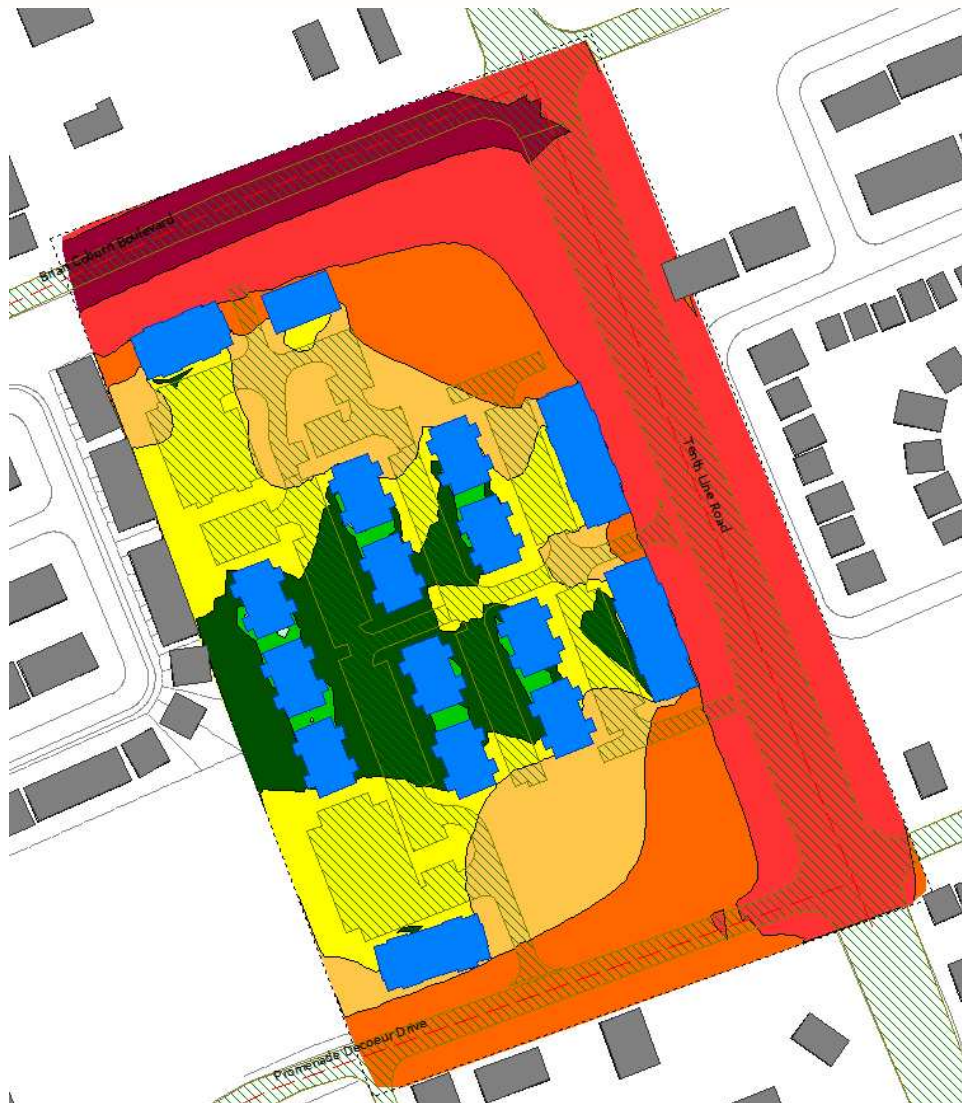
FIGURE 7: NIGHTTIME TRAFFIC NOISE CONTOURS (4.5 M ABOVE GRADE)
