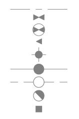
EXISTING WATERMAIN EXISTING VALVE AND VALVE BOX EXISTING VALVE CHAMBER EXISTING REDUCER EXISTING FIRE HYDRANT EXISTING SANITARY MH AND SEWER EXISTING STORM MH AND SEWER EXISTING CATCHBASIN MANHOLE EXISTING CATCHBASIN
