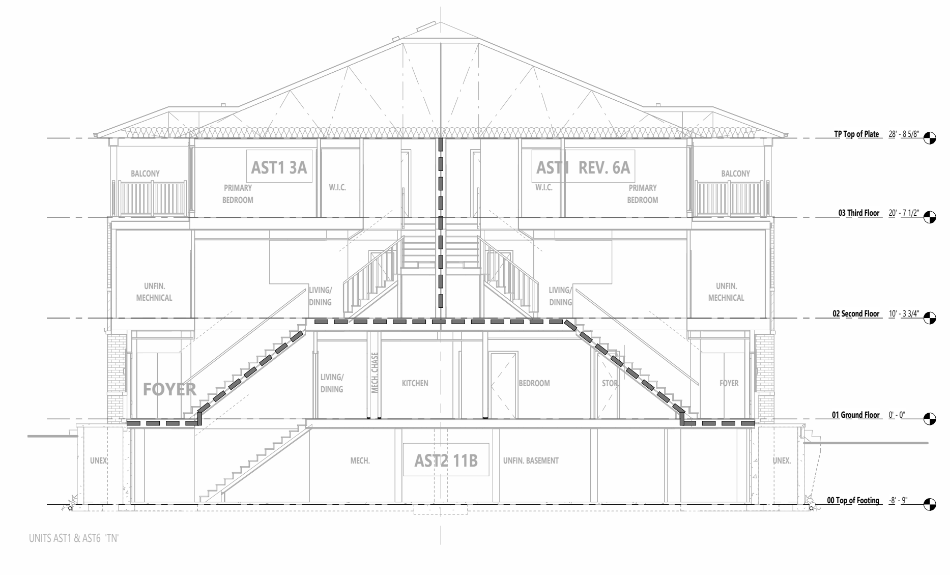
BUILDING SECTION B-B FIRE SEPERATION
