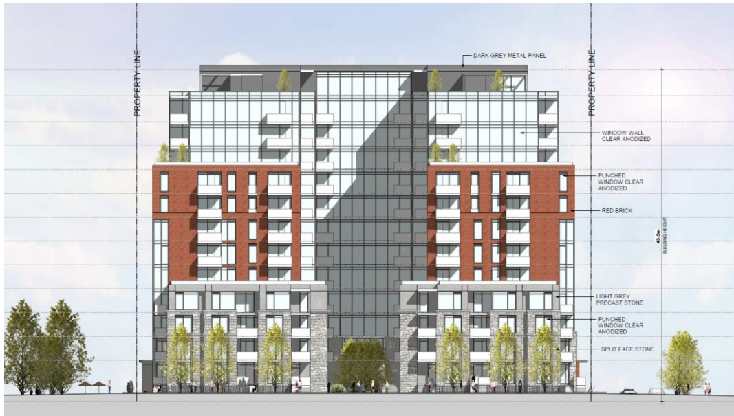
Figure 21: Glass divides the mass into two blocks and lightens the setbacks on the upper floors. Roderick Lahey Architect 2021.
