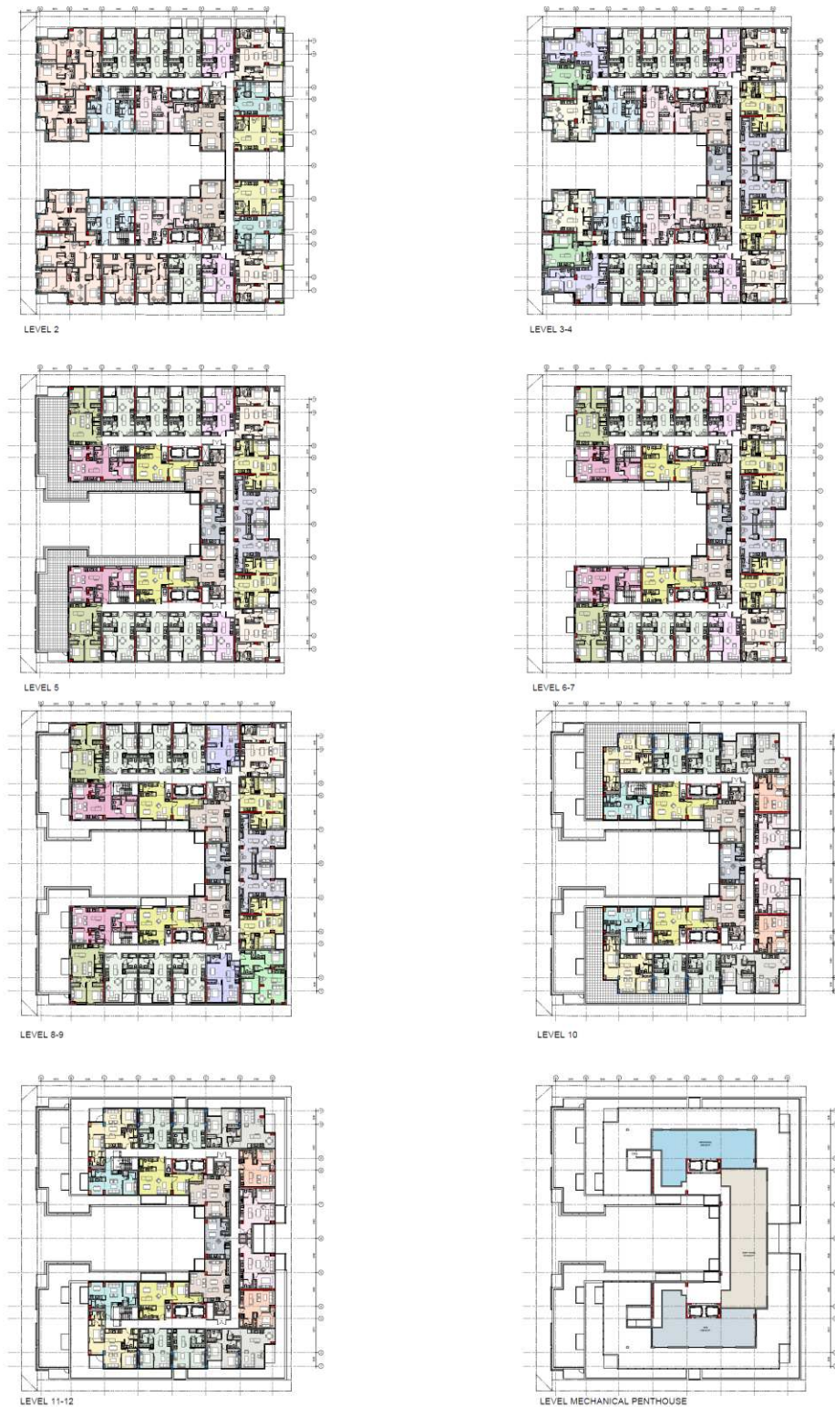
Figure 24: Floor plans L1 through to the 13th floor illustrating the retail and residential components. North (Armstrong Street) is to the left of the image. The proposed plan includes a pedestrian link extending from Wellington Street West through to Armstrong Street. Note the ground floor residential units fronting onto Armstrong. Source: rla Architecture 2021.
