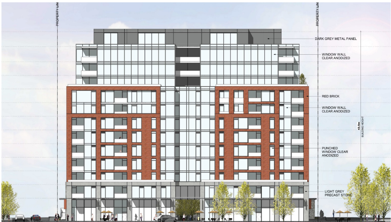
Figure 20: Materiality along Wellington Street West
