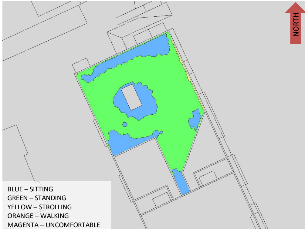
FIGURE 4A: SPRING - WIND COMFORT, LEVEL 6 AMENITY TERRACE (BUILDING A)
