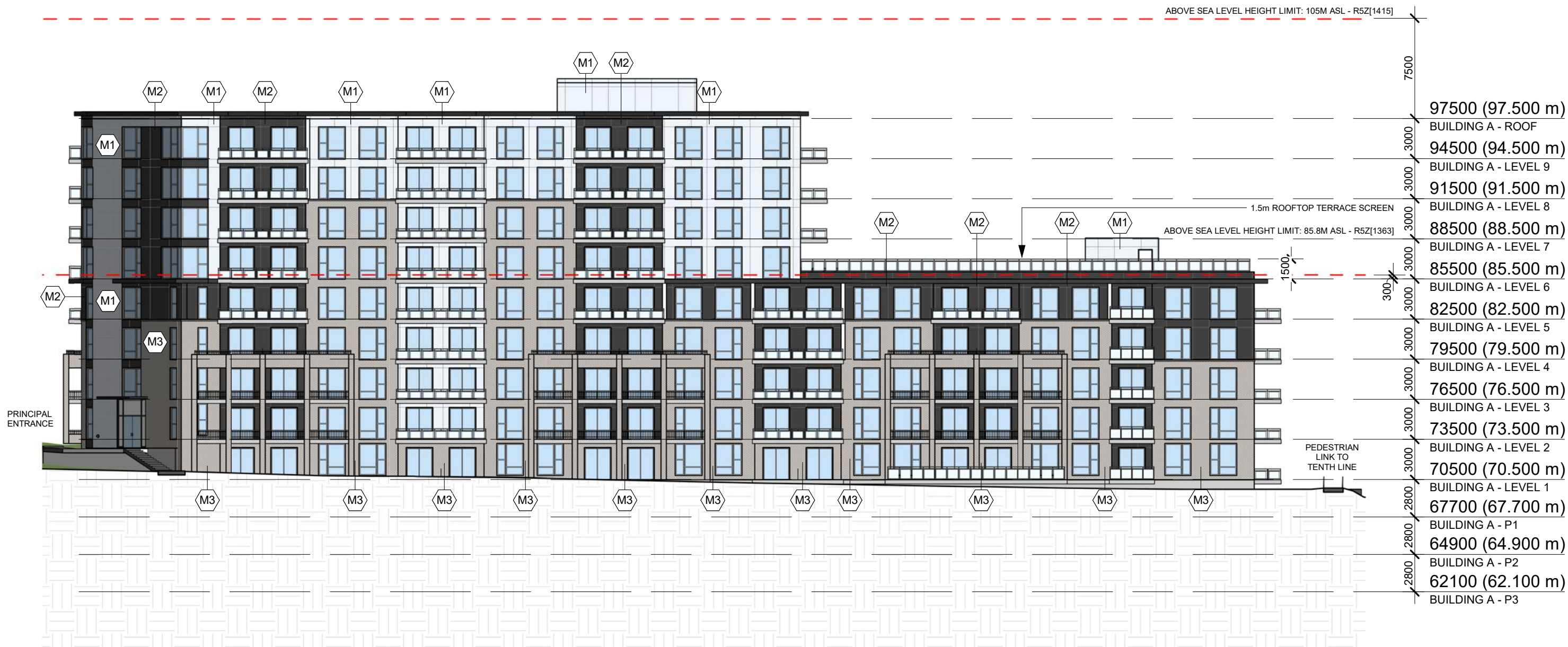
1 BUILDING A - EAST ELEVATION 300 1 : 300
