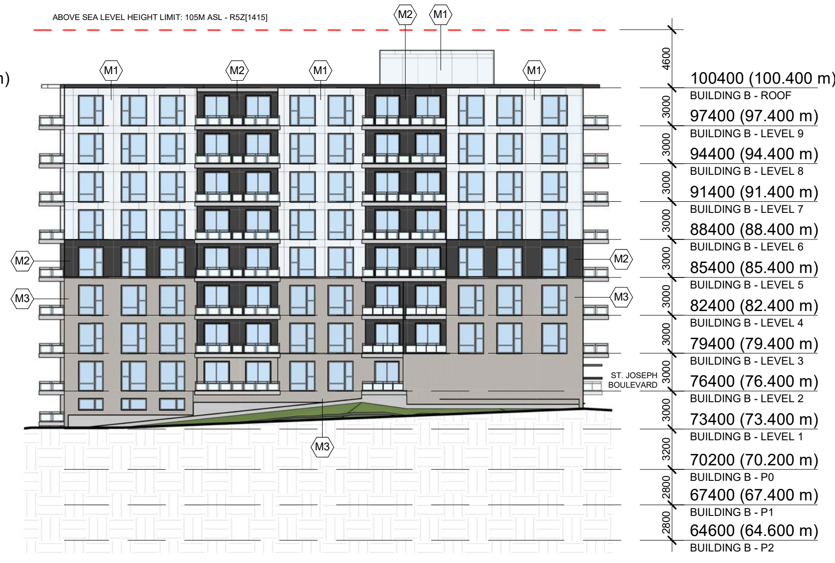
2 BUILDING B - WEST ELEVATION 303 1 : 300
