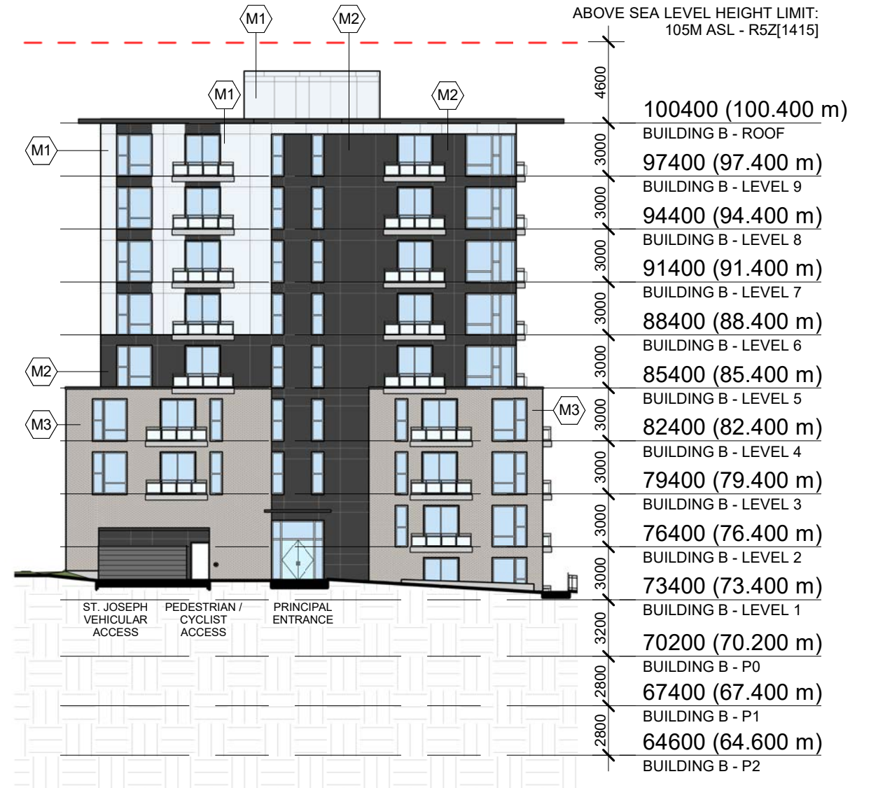
2 BUILDING B - SOUTH ELEVATION 304 1 : 300
