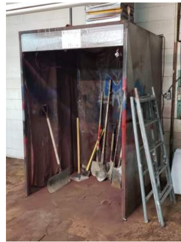
Photo 8: Alternate view of the former spray booth located on the western wall of the northern portion of the Site building.
