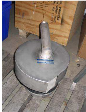
VHV with air vent for minimal slopes
