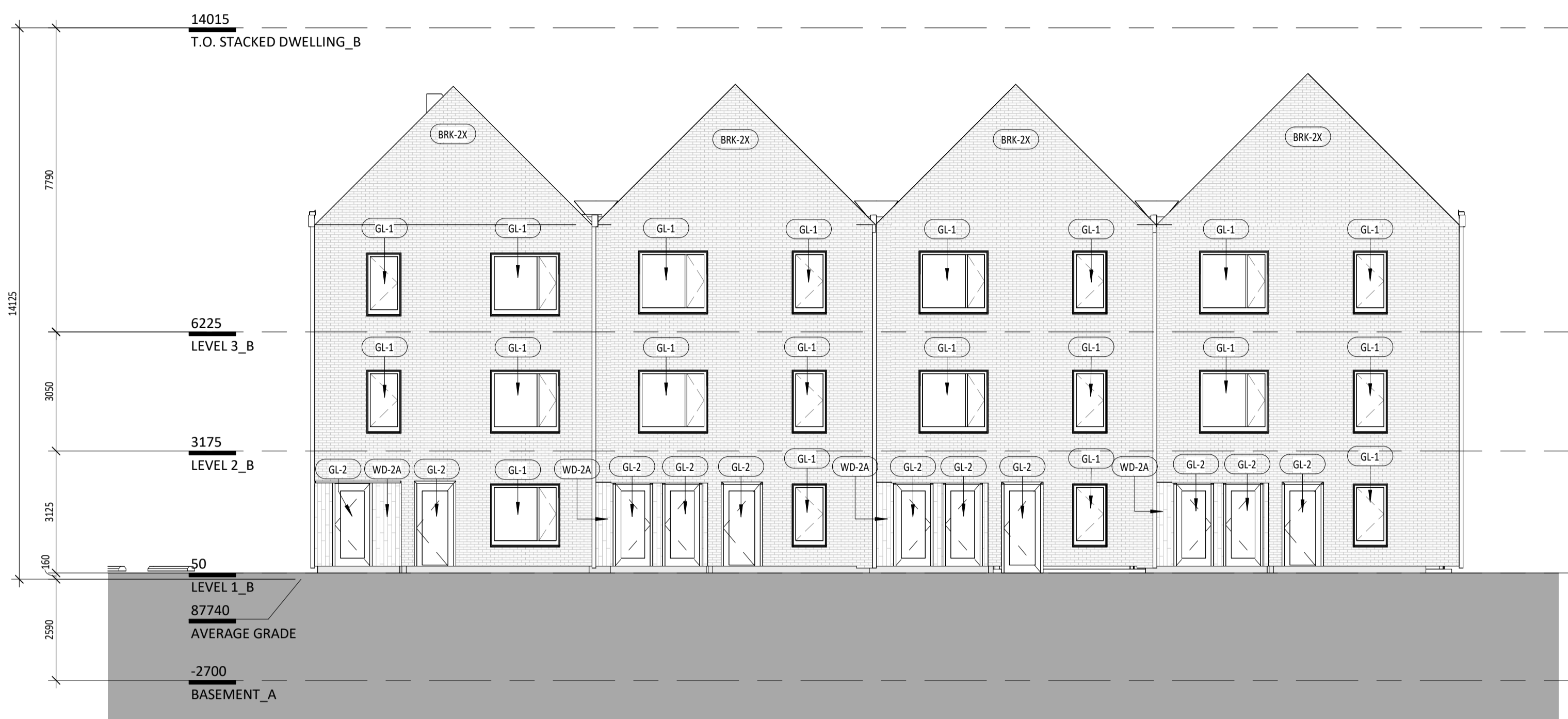
1 BLOCK 4 - NORTH ELEVATION - SPA 1 : 100
