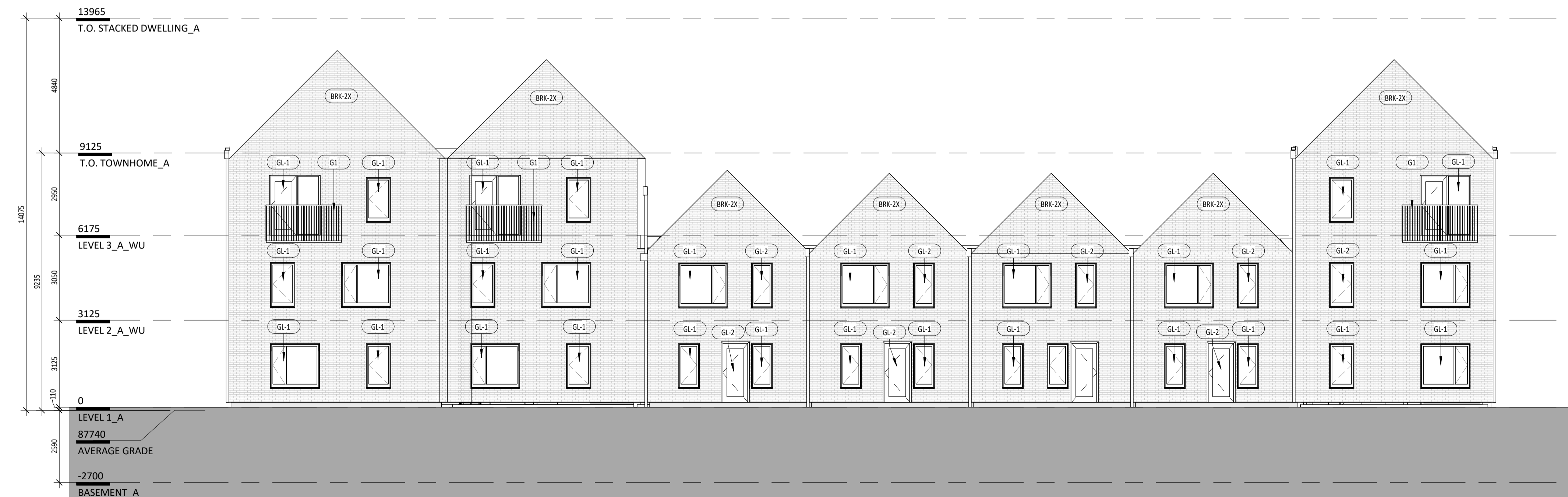
2 BLOCK 2 - SOUTH ELEVATION - SPA 1:100
