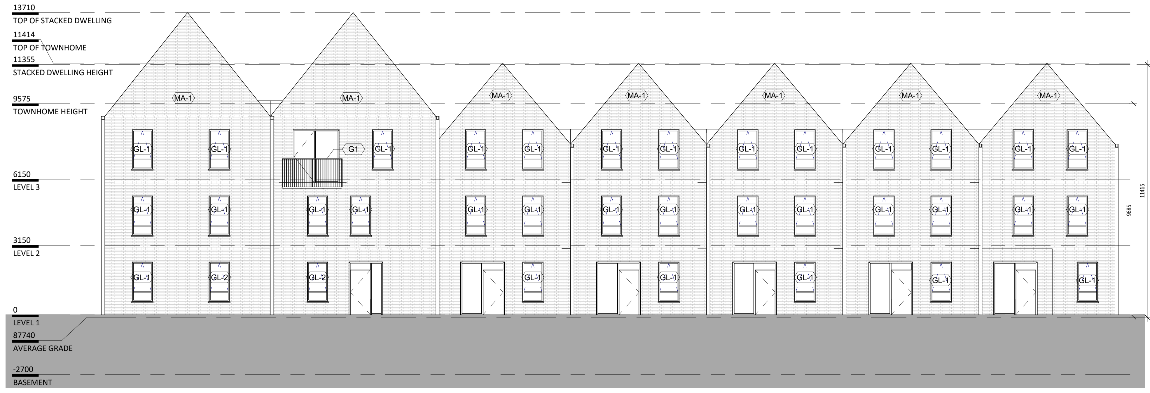
2 BLOCK 3 - SOUTH ELEVATION 1:100
