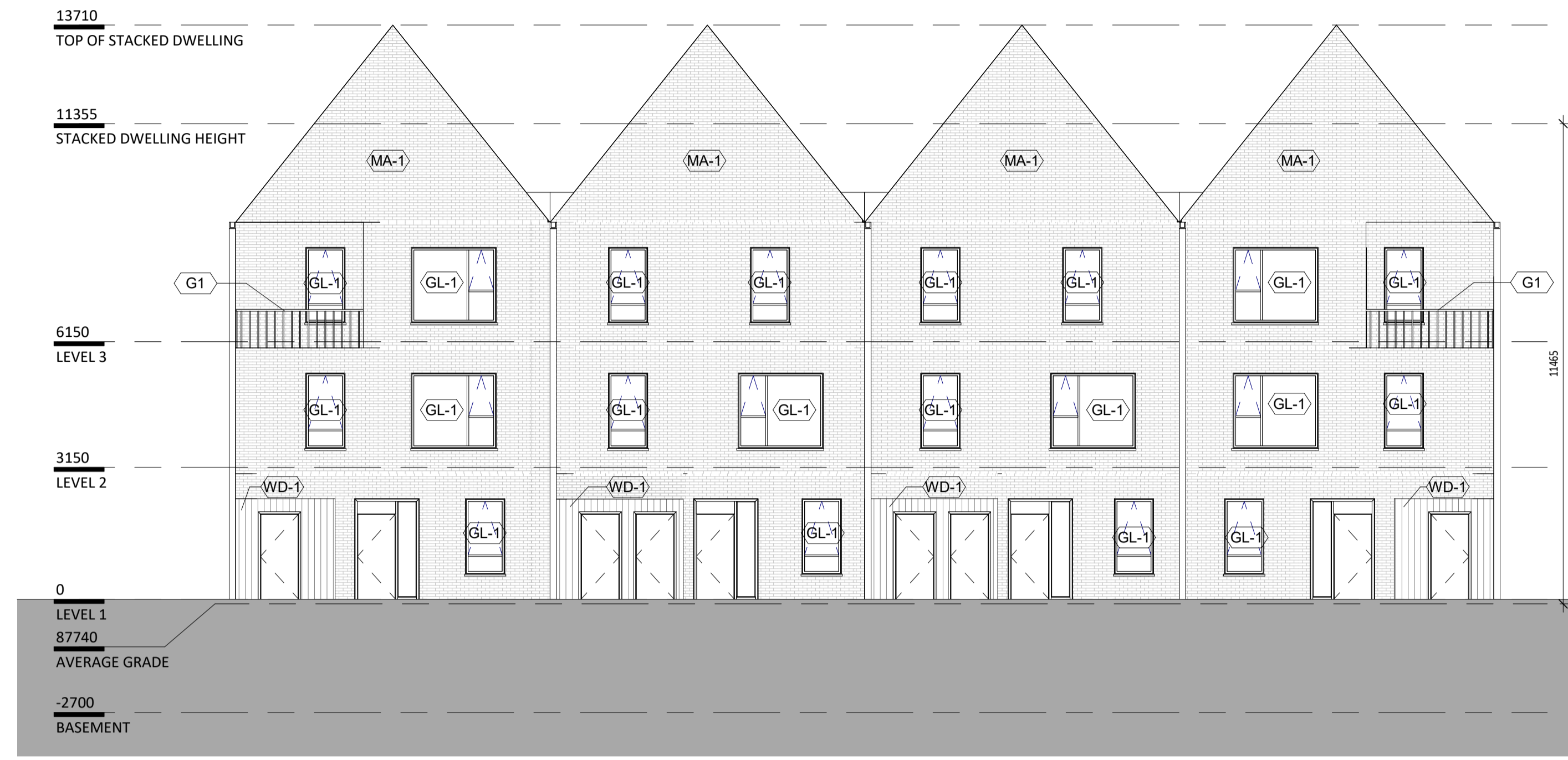
1 BLOCK 4 - NORTH ELEVATION 1:100
