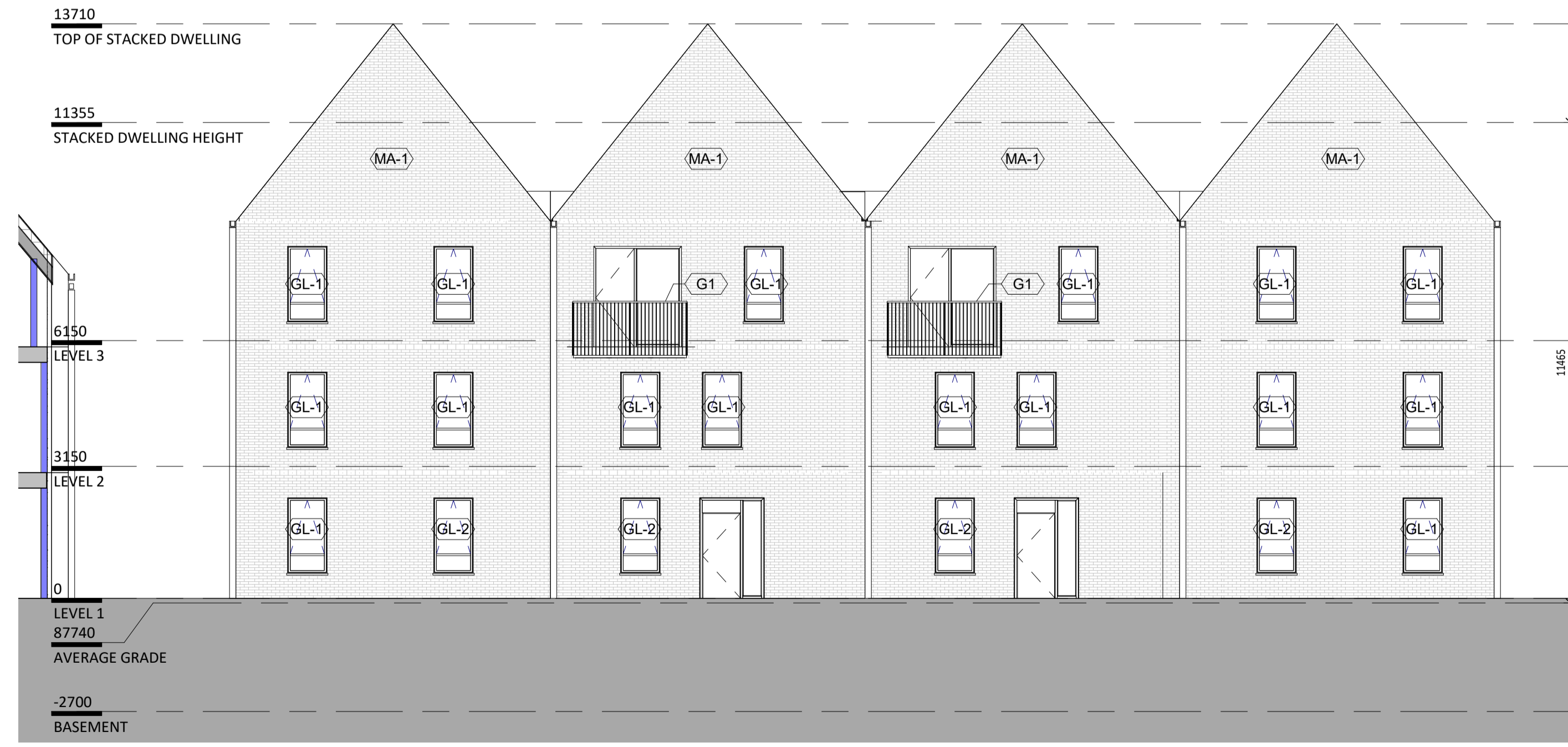
3 BLOCK 4 - SOUTH ELEVATION 1:100
