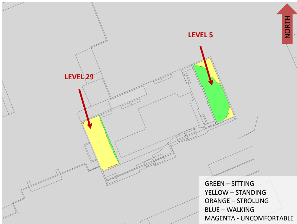
FIGURE 4B: SUMMER – WIND COMFORT CONDITIONS, AMENITY TERRACES
