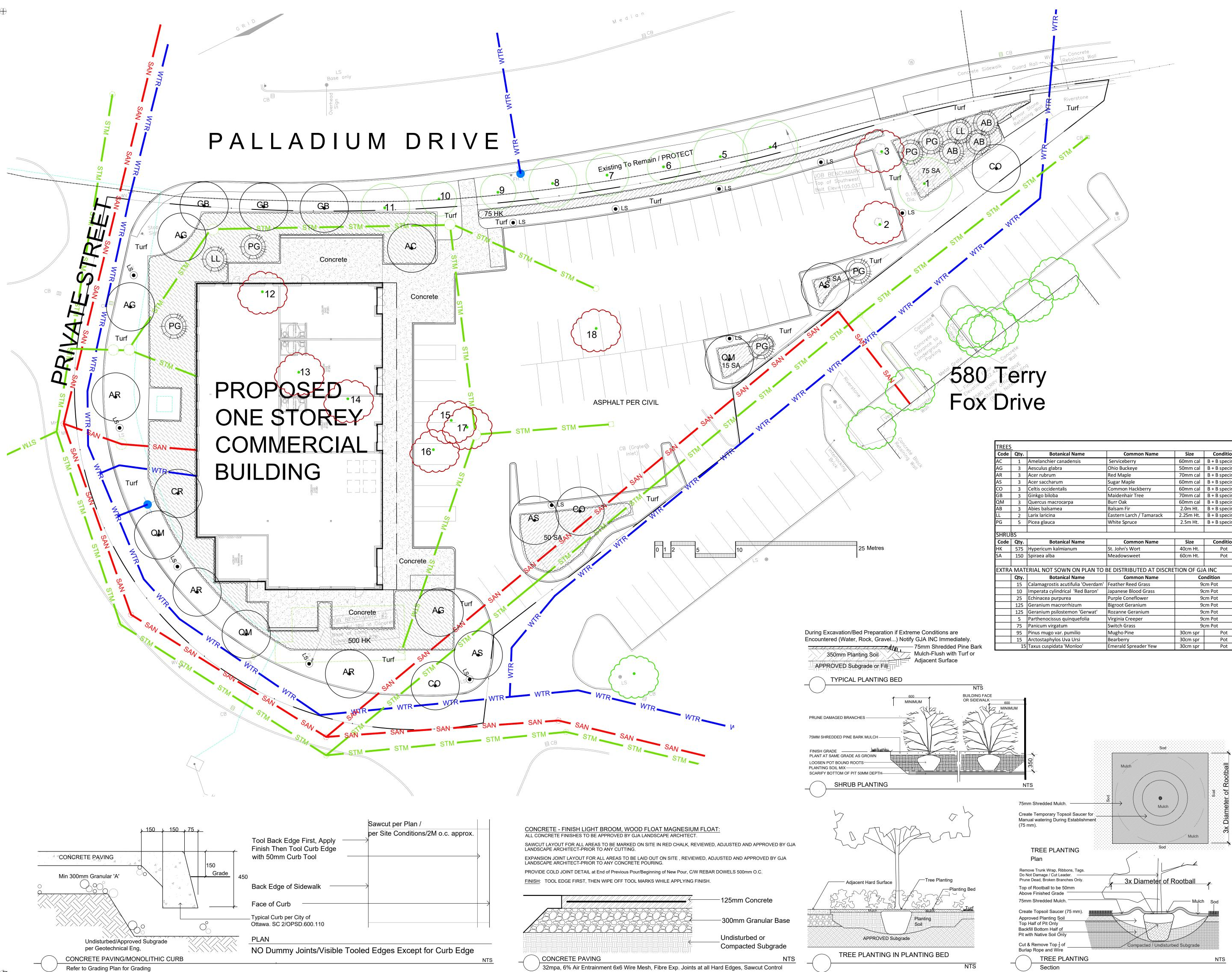
32mpa, 6% Air Entrainment 6x6 Wire Mesh, Fibre Exp. Joints at all Hard Edges, Sawcut Control Joints (1" depth) +-2.0m O.C. as
