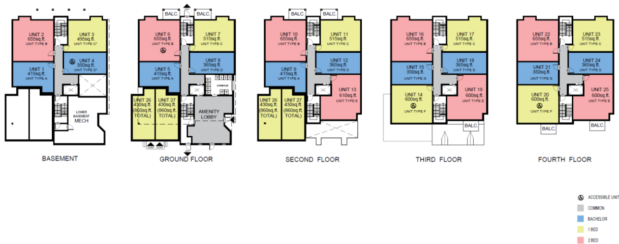
Figure 21: Plan views of the proposed development including the two retained row houses and the infill development behind. The 25 units are colour coded to indicate number of bedrooms. Source: Rosaline Hill Architects Inc. 2022
