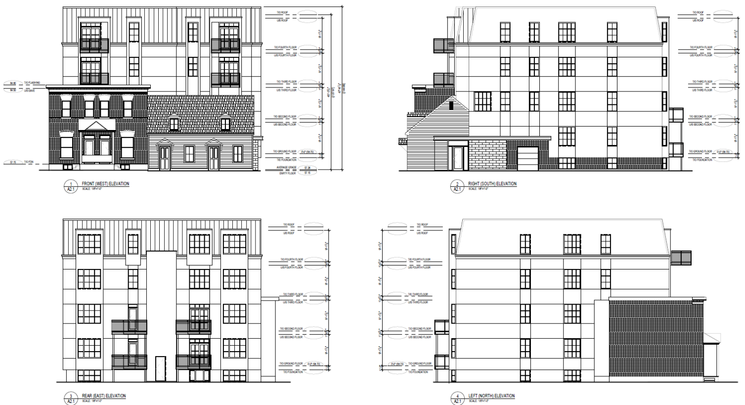
Figure 22: Elevations of the development. Note the modified mansard treatment of the 4 th floor. Source: Rosaline Hill Architects Inc. 2022
