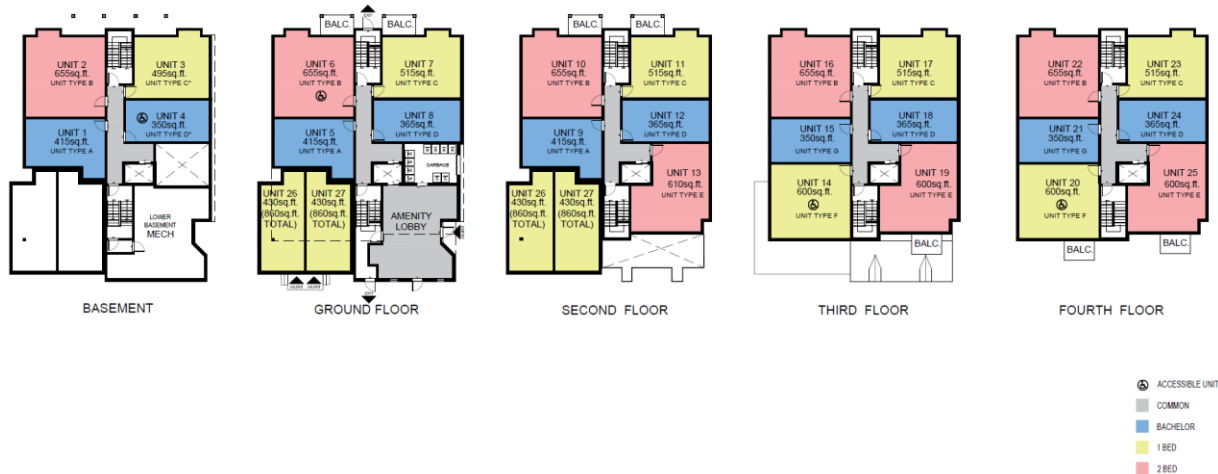
Figure 25: Plan views of the proposed development including the two retained row houses and the infill development behind. The 25 units are colour coded to indicate number of bedrooms. Source: Rosaline Hill Architects Inc. 2022
