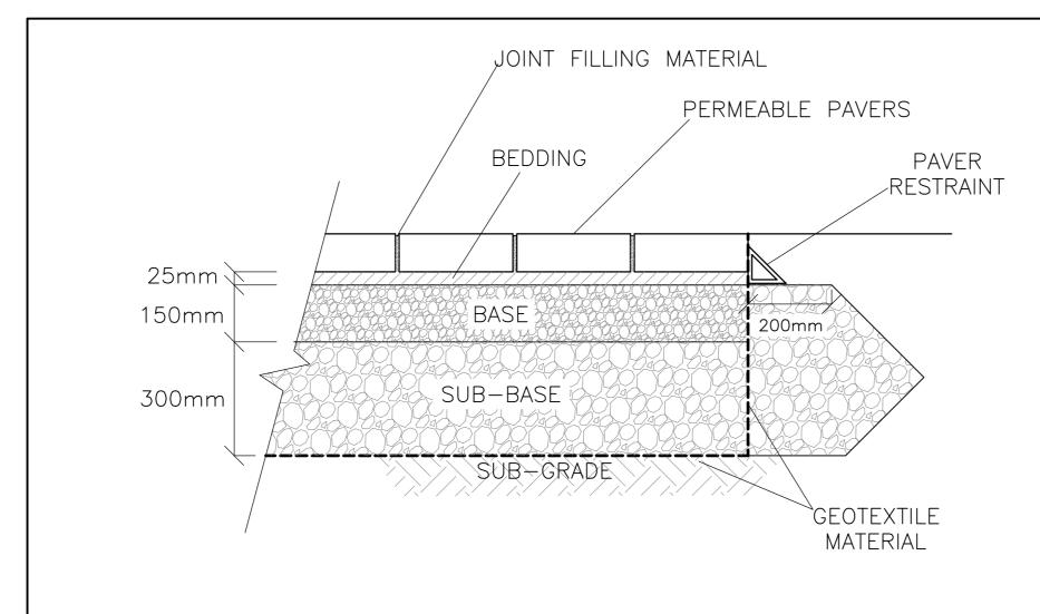
JOINT FILLING MATERIAL: 2.5-10mm AGGREGATE OR AS RECOMMENDED BY MANUFACTURER BEDDING COURSE: 2.5-10mm AGGREGATE OR AS RECOMMENDED BY MANUFACTURER BASE COURSE: 5-28mm AGGREGATE OR AS RECOMMENDED BY MANUFACTURER SUB-BASE COURSE: 40-80mm AGGREGATE OR AS RECOMMENDED BY MANUFACTURER COMPACT EACH LAYER AS RECOMMENDED BY MANUFACTURER
