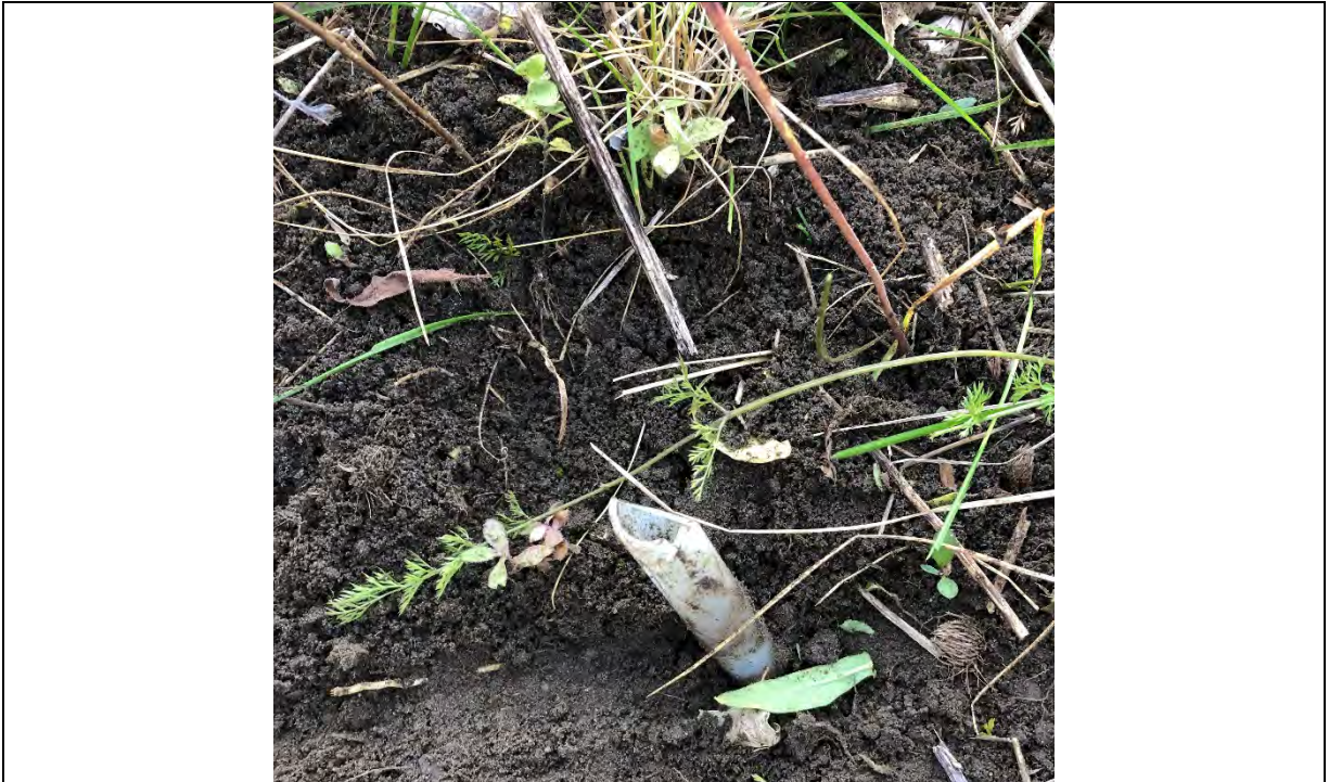
Photo 011 View of Waterra tubing at a destroyed monitoring well location at the Site with no visible well casing, roadbox or monument cover
