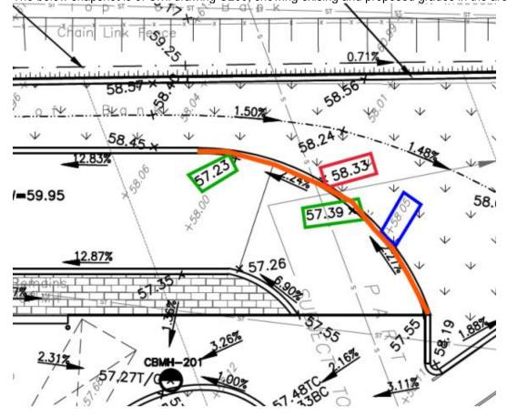
The existing grade elevation over the storm pipe in the location of the retaining wall is approximately 58.05 (Blue), with the finished grade on the high side being approximately 58.33 (Red), and the low grade varies between 57.39 and 57.23 (Green). This results in a maximum retained height of soil of 1.1m
