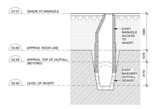
3 SECTION - EXIST. OUTFALL SEWER AT EXIST. BOTELER INVERT
