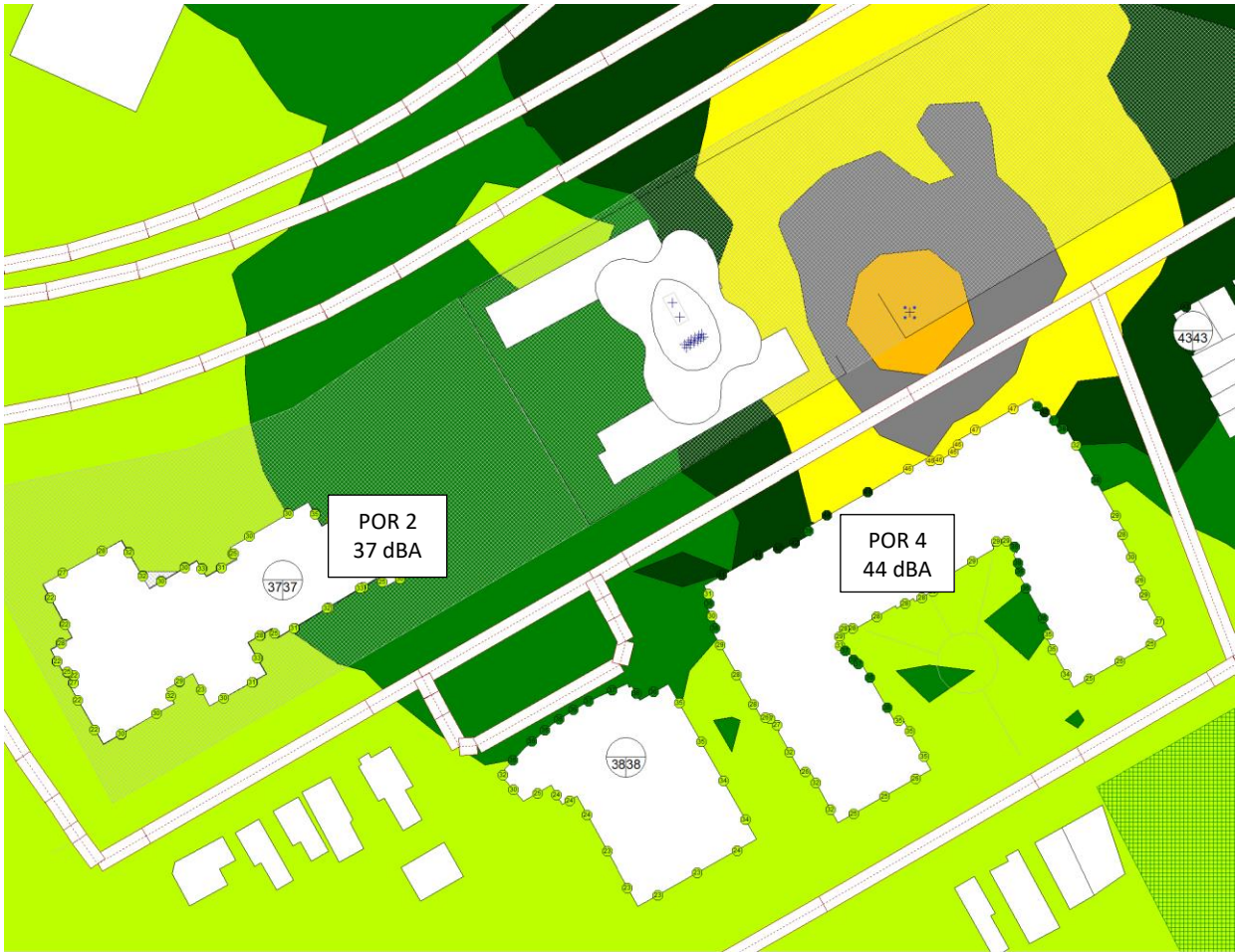
Figure 2.4 – Noise map at 10 m height with current equipment selections for daytime operations, with generator on.
