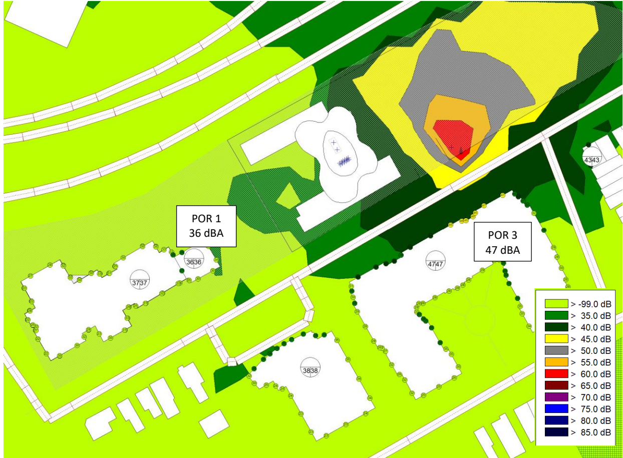
Figure 2.3 – Noise map at 1.5 m height with current equipment selections for daytime operations, with generator on.
