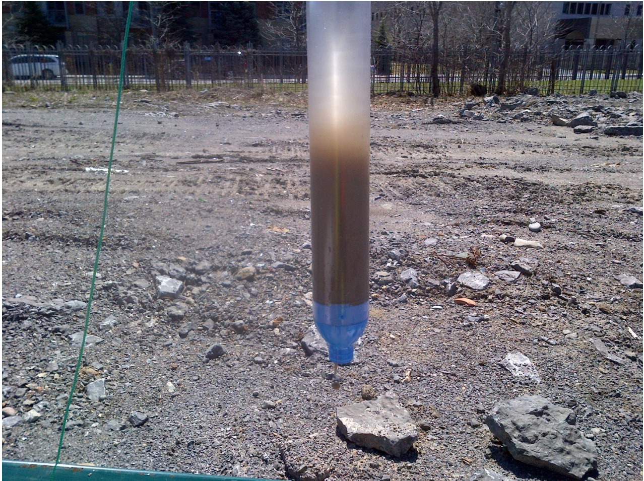
Photo 5: View of sediment present in sampling bailer of collected water from MW14-1 on April 24, 2014.
