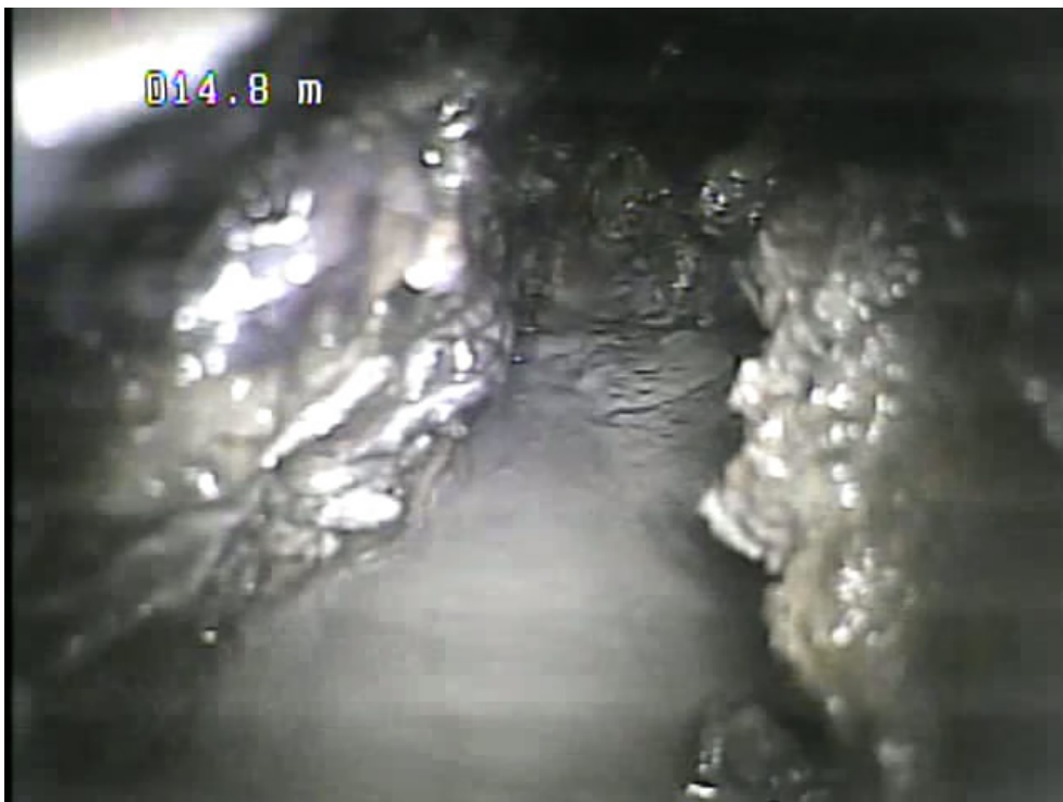
Photo 4: View of karst feature, depth 14.4 m BGS. Sediment filled water visible at bottom of photo.
