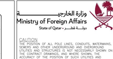
THE POSITION OF ALL POLE LINES, CONDUITS, WATERMAINS, SEWERS AND OTHER UNDERGROUND AND OVERGROUND UTILITIES AND STRUCTURES IS NOT NECESSARILY SHOWN ON THE CONTRACT DRAWINGS, AND WHERE SHOWN, THE ACCURACY OF THE POSITION OF SUCH UTILITIES AND STRUCTURES IS NOT GUARANTEED. BEFORE STARTING WORK, DETERMINE THE EXACT LOCATION OF ALL SUCH UTILITIES AND STRUCTURES AND ASSUME ALL LIABILITY FOR DAMAGE TO THEM.
