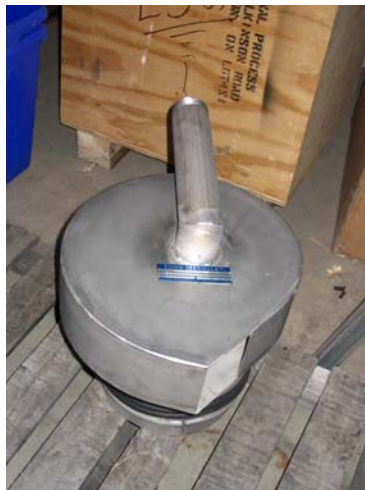
VHV with upstream air vent (applications where outlet pipe is > 80% full at peak flow)
