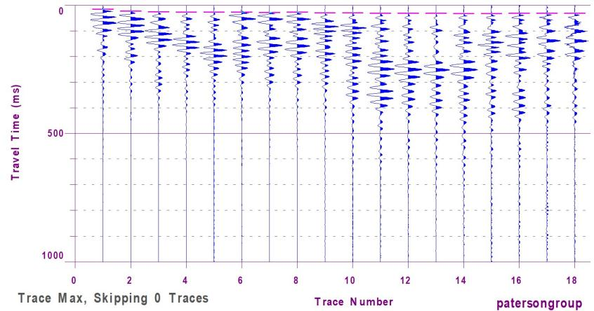
Figure 2 – Shear Wave Velocity Profile at Shot Location -1.5 m
