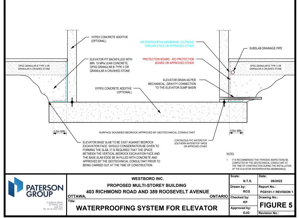
p:\autocad drawings\geotechnical\pg51xx\pg5101\pg5101- fig 5 - waterproofing systems for elevator.dwg
