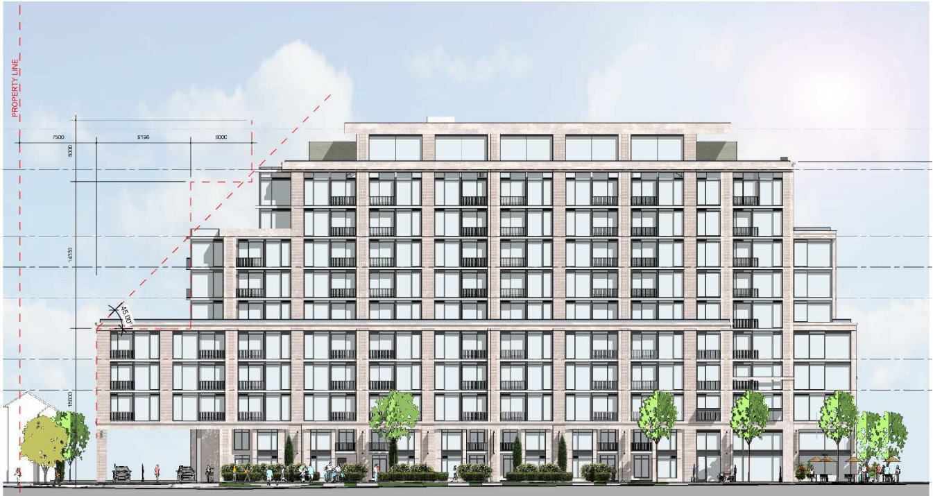
Figure 7: West Elevation Showing 45 Degree Angular Plane
