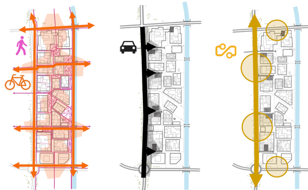
Figure 1. Design Principles for Pedestrians, Cyclists, Cars and Public Transport (Mobility Concept for Merwede, Utrecht)
