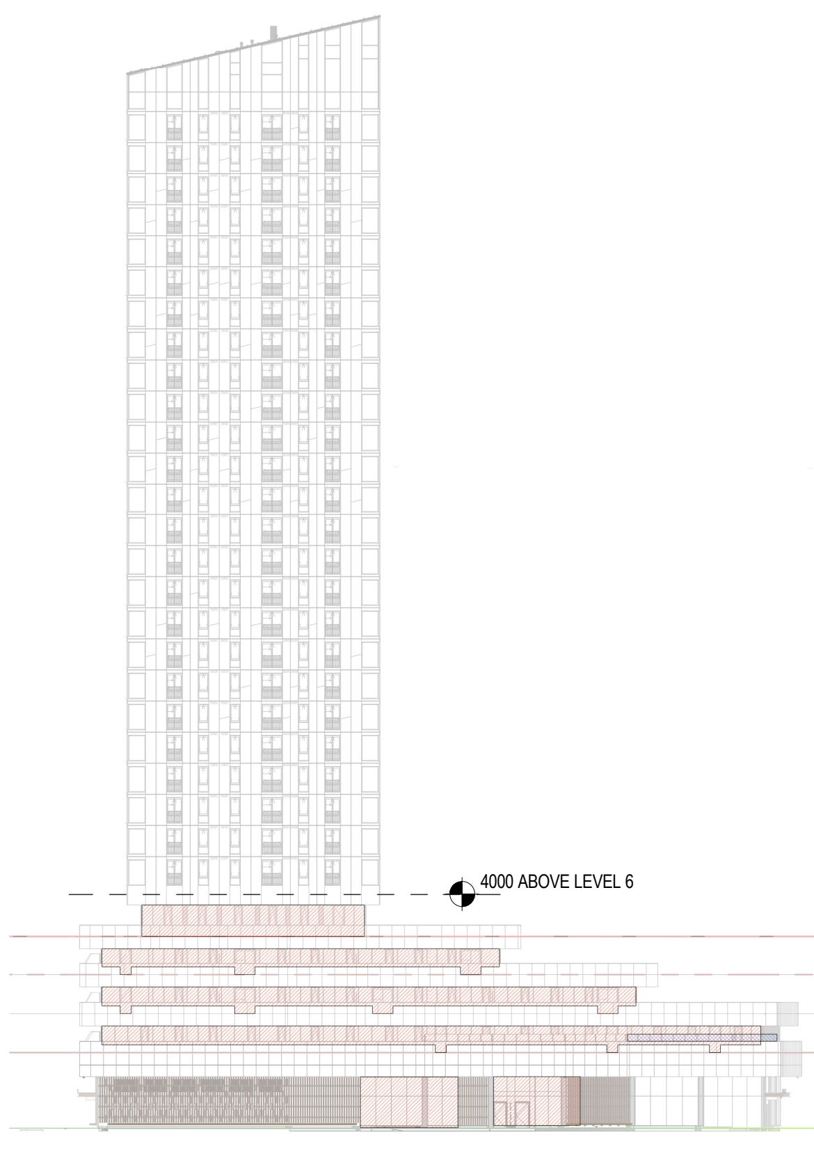
3 BIRD COLLISION DETERRENCE - EAST BUILDING - NORTH ELEVATION 1:500
