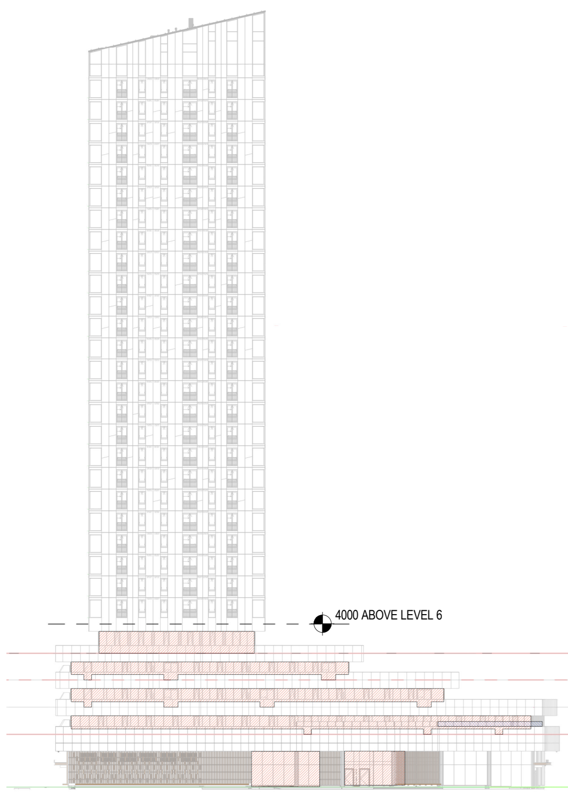
3 BIRD COLLISION DETERRENCE - EAST BUILDING - NORTH ELEVATION 1:500
