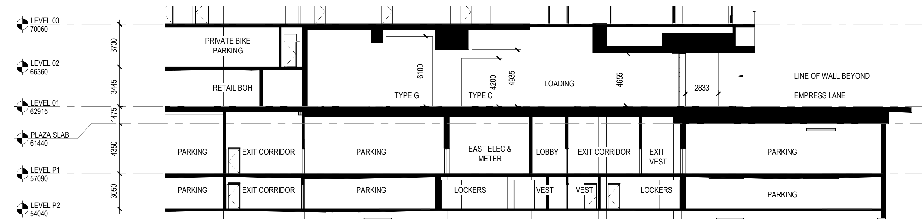
① PARTIAL SECTION @ LOADING DOCK ACCESS 1 : 200
