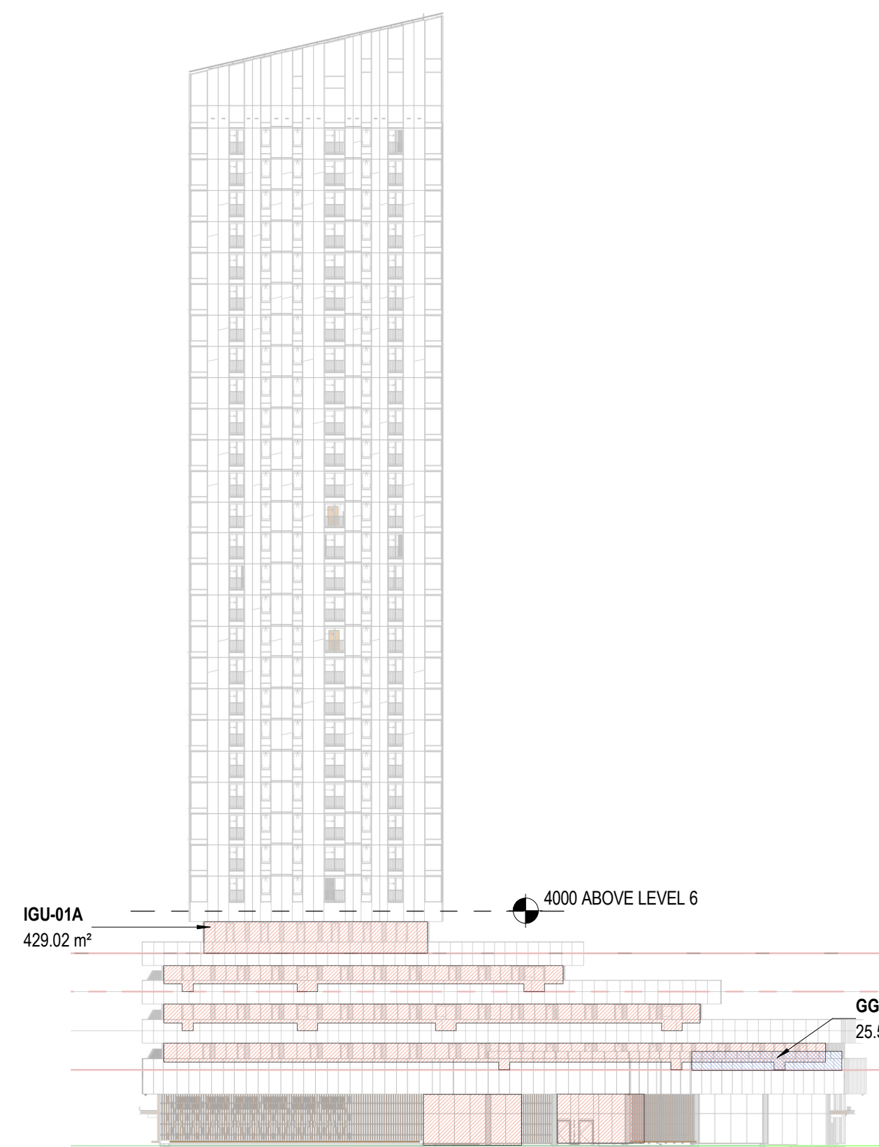
3 BIRD COLLISION DETERRENCE - EAST BUILDING - NORTH ELEVATION 1 : 500
