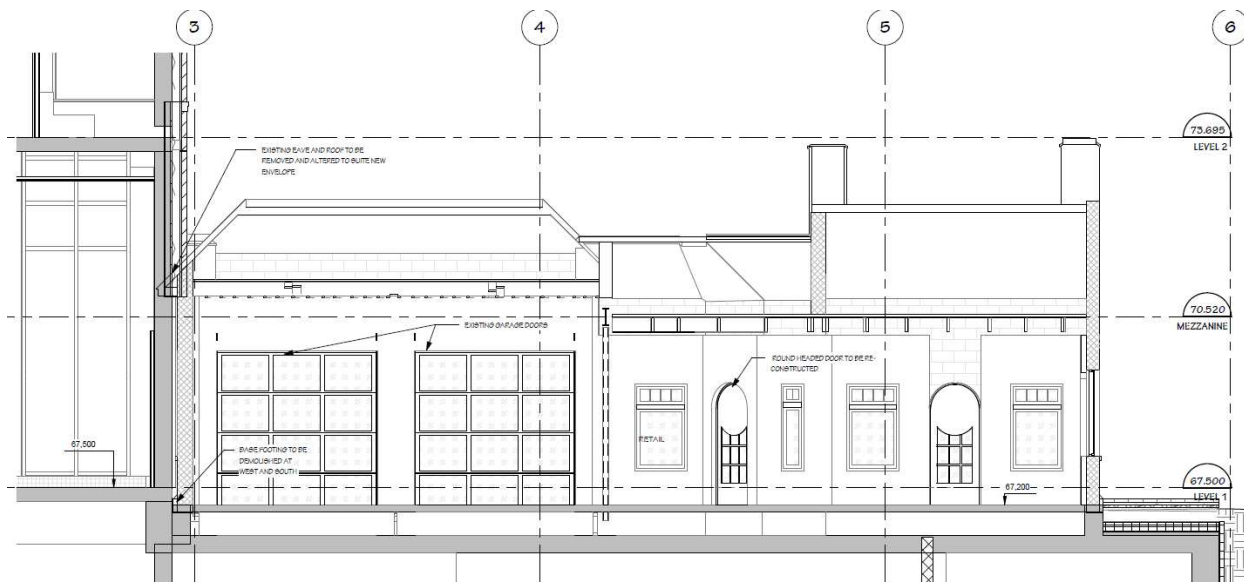
HERITAGE SECTION 2-LOOKING NORTH 72 / SCALE: 1/40
