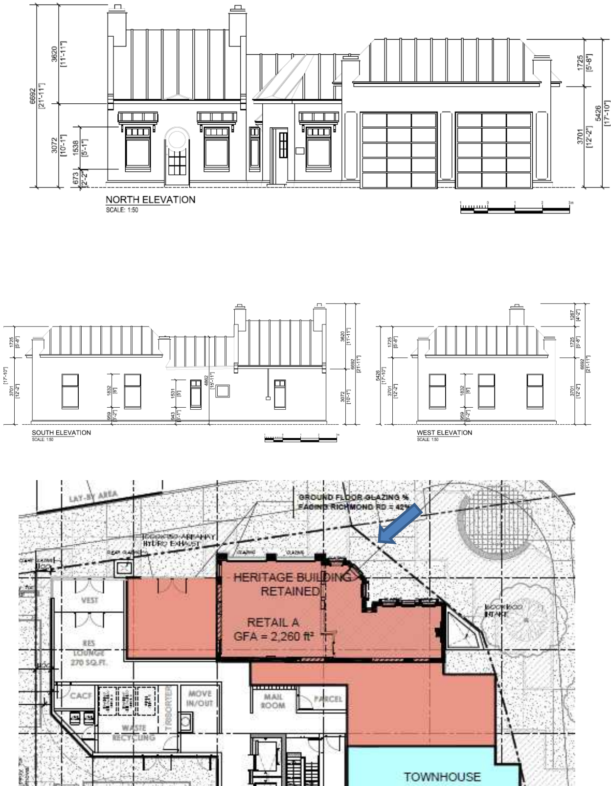
Figure 7: Context plan illustrating the heritage building incorporated into Retail A (pink) with a GFA 2,260 sf. The hatched lines delineate the portion of the walls to be removed and suggests that the two spaces will be united. The south and west walls will be retained with the introduction of doors to link to the mid-rise. As-found plans have been completed. The property lines are delineated with dashed lines and are noted with an arrow.
