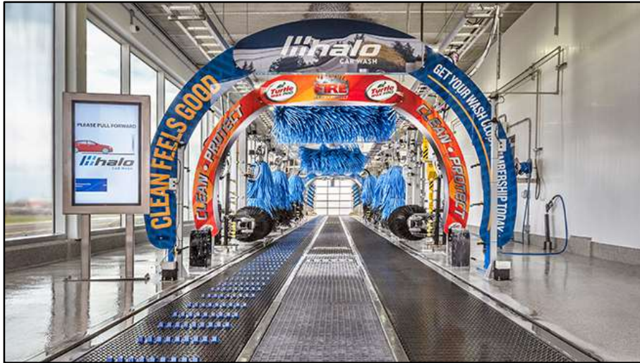
Exhibit L: Interior of typical Halo Car Wash tunnel with double-conveyor belt system
