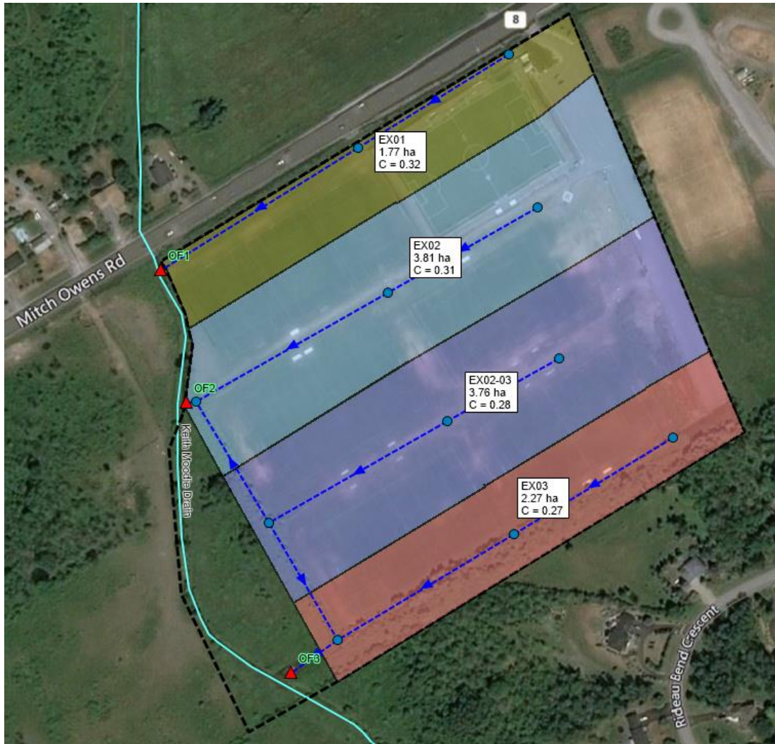
Figure 2: Existing Conditions Catchment Areas and Runoff Coefficients
