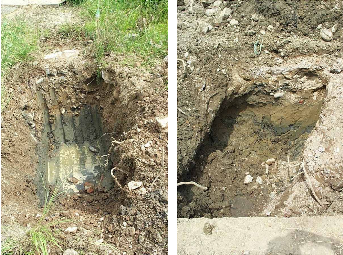
FIG. 4-27: Photographs of test pits for vane shear tests VST-3 and 4 that show the characteristics of the surface fill and underlying fine-grained soils. (source: http://peer.berkeley.edu/lifelines/research_projects/3A02/ )
