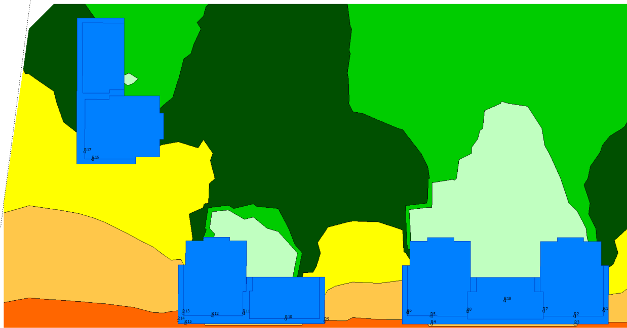
FIGURE 5: NIGHTTIME TRAFFIC NOISE CONTOURS (10 M ABOVE GRADE)
